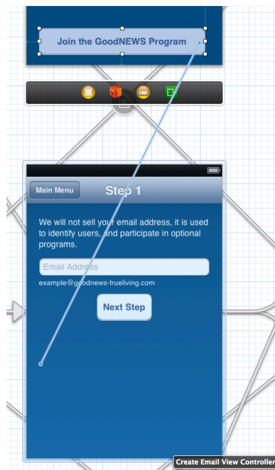
Figure 5.1 Connecting a Segue to a button push, just control + click on the button and drag to the corresponding view controller.
